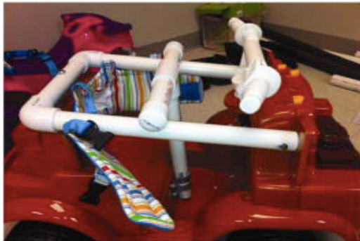
Figure 4 Roll cage on a ride-on-car with PVC pipes
